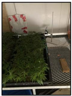
Figure 2 Using the Apogee SQ-640 Light Pollution Sensor and  $\mu$ Cache Bluetooth Micro Logger (hidden behind green sensor base) on a retort stand to directionally-characterize stray light pollution in cannabis photoperiod treatment plots.
